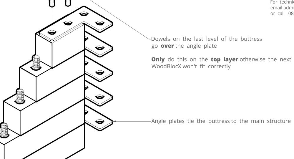
WoodBlocX buttresses act as cantilevers with the weight of soil pushing down on them to keep the main structure supported.
